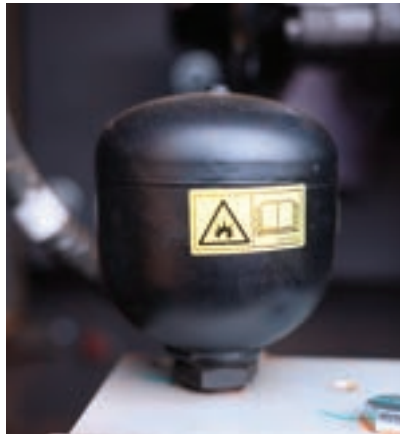
Boom Accumulator For the safe lowering of boom in the event of power loss.
