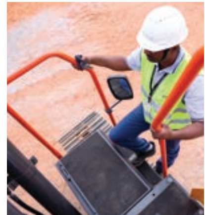
Side access New improved coloured 3-point side access enhances safety and ease to access.
