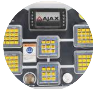
USER FRIENDLY DASHBOARD HMI - Control system, Electrical CAN Bus System
