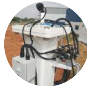
PROPORTIONAL VALVE BLOCKS for Steering, slewing & leveling, 4 LED lamps (2900 lumens) on all four columns as standard
