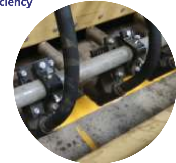
ELECTRICAL VIBRATORS for consolidation of concrete
