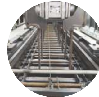
DOWEL BAR INSERTER Dowel bars are used for increasing load transfer efficiency between two slabs
