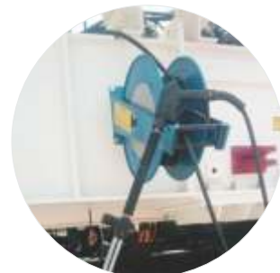
CLEANING SYSTEM High pressure water cleaning system with 20m Hose reel
