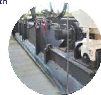
OSCILLATION CORRECTION BEAM Oscillating movement for removing the irregularities caused by Dowel bar Insertion
