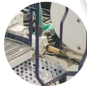
LOW PRESSURE WATER PUMP for filling water tank.
