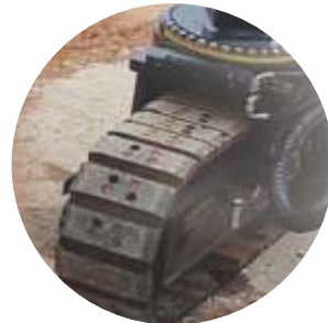
TRACK WITH SLEWING DRIVE Slewing drive for steering of tracks. Tracks fitted with Highly wear resistant polyurethane pads
