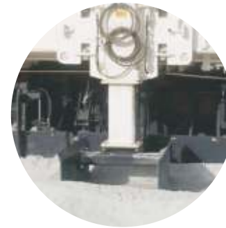
SPREADER PLOUGH for spreading of concrete
