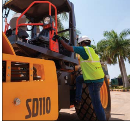
3-Point Contact Handrail
