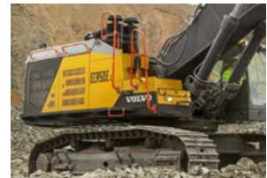
Access way with Handrail
