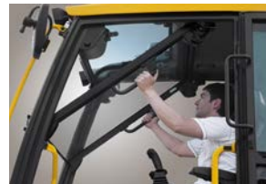
Pull-up type openable front upper window & removable front lower window
