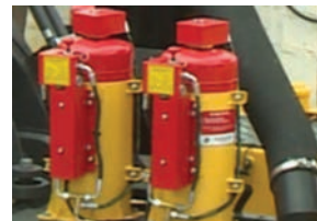
Automatic Fire Detection & Suppression System (AFDSS)
