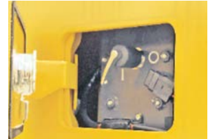
Battery cut-off switch
