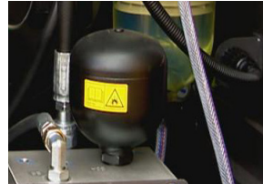
Accumulator for Boom lowering
