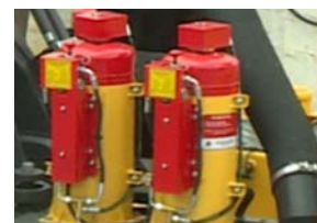
Automatic Fire Detection & Suppression System (AFDSS)
