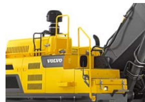
Access way with Handrail
