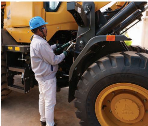
Ground level access of all lubricating points with extended metal pipes
