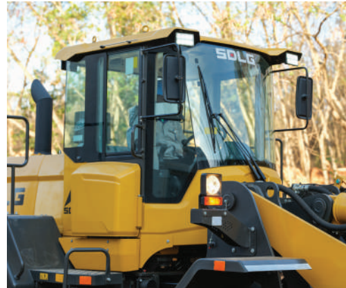
Extra Working lights, reverse horn, and rotating beacon for better visibility
